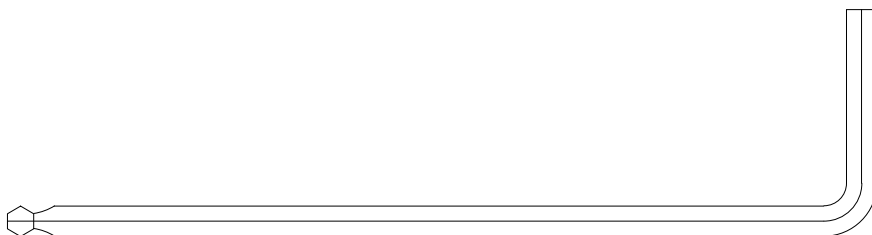
H9 (x1) Allen Key/Clé Allen/Llave Allen 3/16 x 4 5/16 in 4 x 110 mm
