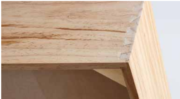
Drawer corner blocks and English dovetailed joints
